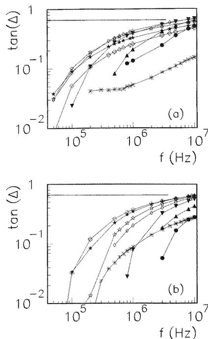
FIG. 8. Loss angle tangent vs frequency for the samples of Fig. 6, at  $T=20^\circ\text{C}$  (a) and  $T=25^\circ\text{C}$  (b), respectively. The line with constant  $\tan\Delta=0.65$  is drawn. For clarity of the picture, the points affected by electrode polarization at  $\phi=0.600$  and 0.515 are not reported. The symbol meanings are as in Fig. 6.
