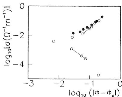
FIG. 4. Experimental values of Fig. 3 arranged to show the linear trend of the  $\log_{10}(\sigma)$  vs  $\log_{10}|\phi - \phi_p|$  below (bottom curve) and above (upper curves) the percolation threshold. The straight lines represent the fitting results. The symbol meanings are as in Fig. 3.
