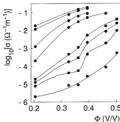
FIG. 2. Experimental  $\sigma(\phi)$  values at different temperatures. From bottom to top in the picture:  $T=10, 15, 18, 20, 28, 32, 38,$  and  $40$  °C. The curves show the crossing of  $\phi_p$  threshold (sigmoidal shape curve) at 15, 18, and 20 °C, the trend above  $\phi_p$  at higher temperatures (upper part of the sigmoidal shape curve) and the trend below  $\phi_p$  at the lowest temperature. The lines are guides for the eyes.
