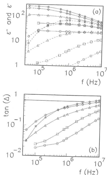
FIG. 9. Real (continuous lines) and imaginary (dashed lines) part of the complex dielectric constant (a) and loss angle tangent (b) vs frequency, for the sample with  $\phi=0.462$  at the temperatures:  $-0.7^\circ\text{C}$  (points),  $6.1^\circ\text{C}$  (squares),  $11.1^\circ\text{C}$  (triangles),  $14.0^\circ\text{C}$  (crosses), and  $16.9^\circ\text{C}$  (stars). The line is  $\tan\Delta=0.65$ .
