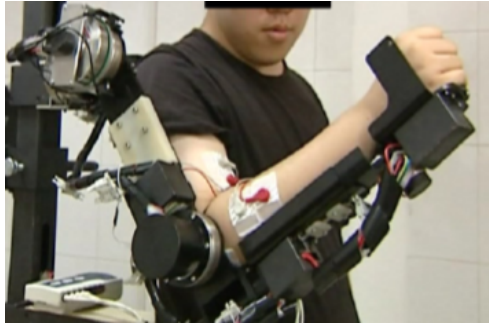
Figure 11: Upper Limb Robotic Exoskeleton Using Biological Signals [9]
