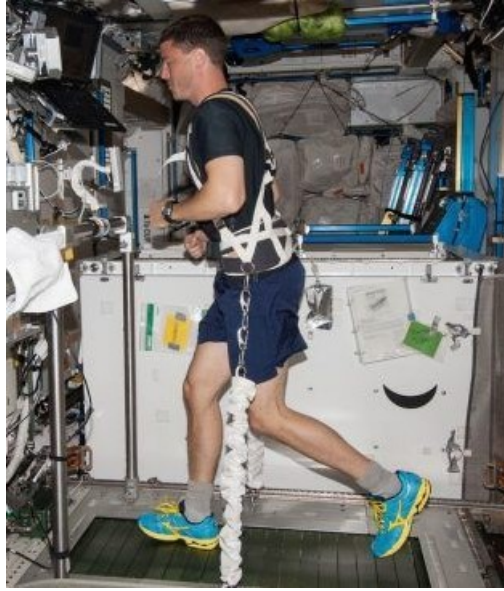
Figure 9: Treadmill with Vibration Isolation and Stabilization (TVIS)
