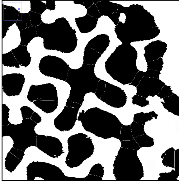
Figure 14. Typical example depicting the watershed and particle area cut-off procedure of a binary image.
