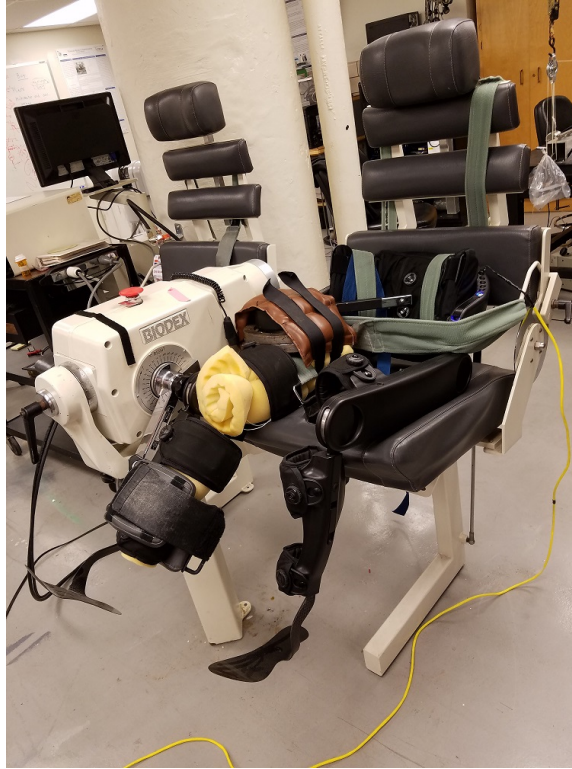
Figure 45: Experimental test setup for the isometric and isokinetic exercises, where the Indego is secured to the Biodex-2 via straps and weights. Foam was added inside the leg braces of the Indego's leg to add shape
