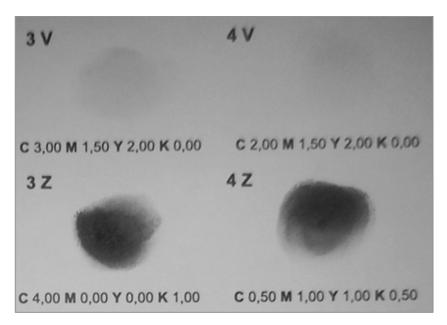
Figure 47. Dye twins 3V, 3Z and 4V, 4Z for offset printing in the IR spectrum at 1000nm
