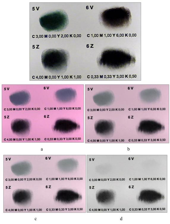
Figure 54. Display of barrier cuts at 570nm, 695nm, 715nm and 850nm of twin dyes 5V and 5Z, 6V and 6Z
