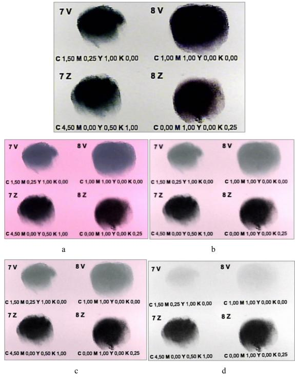
Figure 55. Display of barrier cuts at 570nm, 695nm, 715nm and 850nm of twin dyes 7V and 7Z, 8V and 8Z
