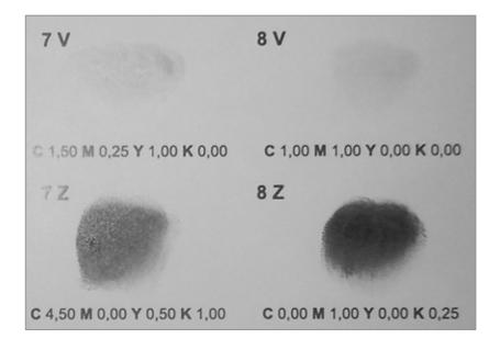
Figure 51. Dye twins 7V, 7Z and 8V, 8Z for offset printing in the IR spectrum at 1000nm
