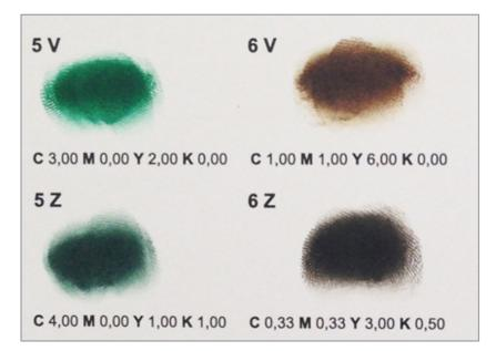
Figure 48. Dye twins for offset printing in the visual spectrum, twin dyes 5V, 5Z and 6V, 6Z
