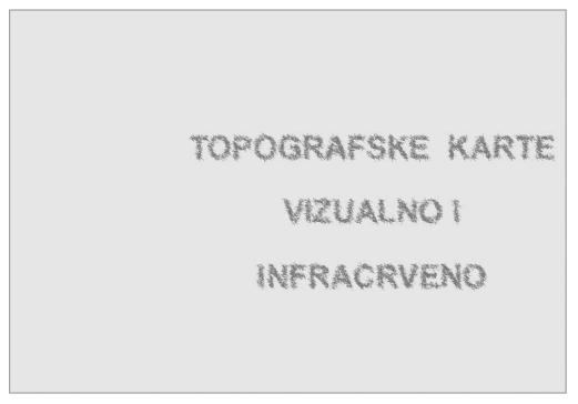
Figure 68. Planned hidden text rasterised with needle raster, Z image at  $1000 \mathrm{nm}$
