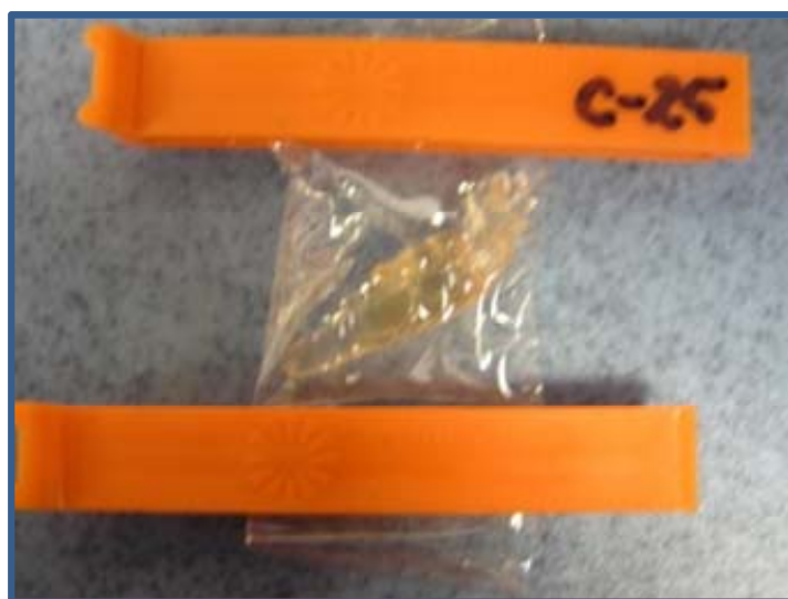
Figure 5.2. TB-Hydrogel Plug in Dialysis Tubing Prior to Gd-DTPA -2 Bath Equilibration.
