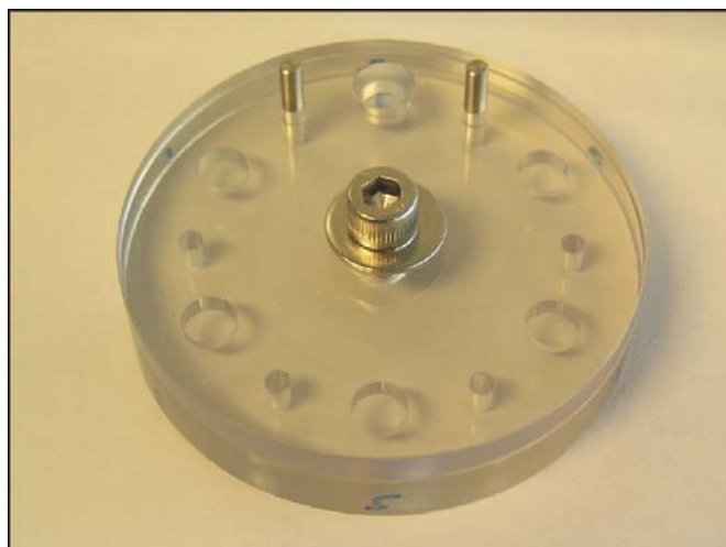
Figure 2.2. Custom Built Confined Compression Testing Apparatus. Wells measured 7.1 mm in diameter and 3 mm in thickness.
