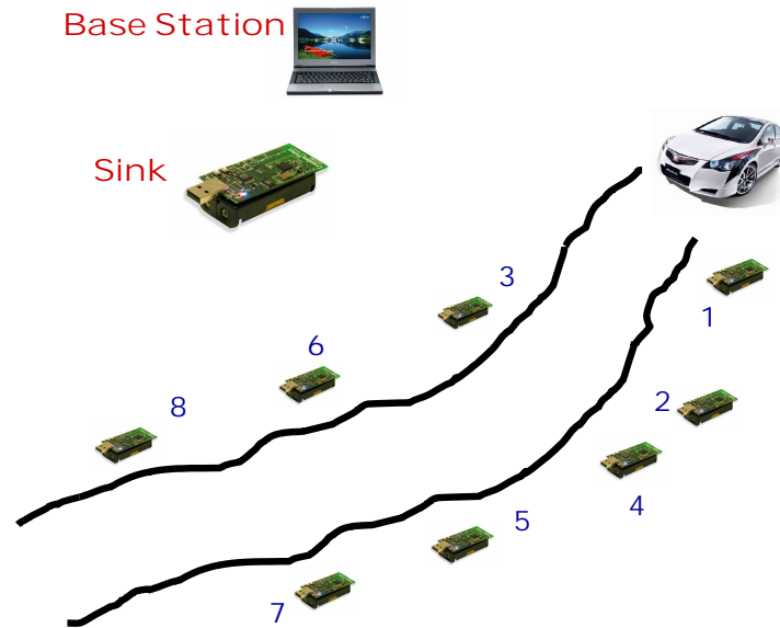
Figure 3: Shows the deployment of wireless sensor network for traffic monitoring application.
