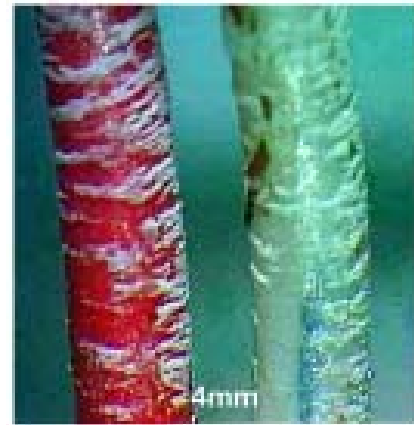
Figure 8.3A: Checking and crazing of the parylene and silastic coating on the wires leading to the ventral plate.
