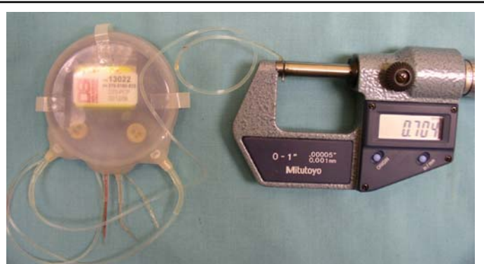
Figure 4.1: The DSI telemetric pressure transducer housing two pressure sensors within the fluid-filled catheters, with one catheter being compressed to a measured displacement to demonstrate the catheter compliancy.
