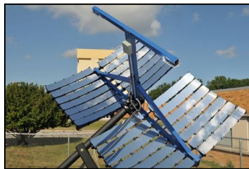
Figure 9: Solar concentrator installation utilizing VMJ photovoltaic cells at NASA GRC [reproduced from source 14]
