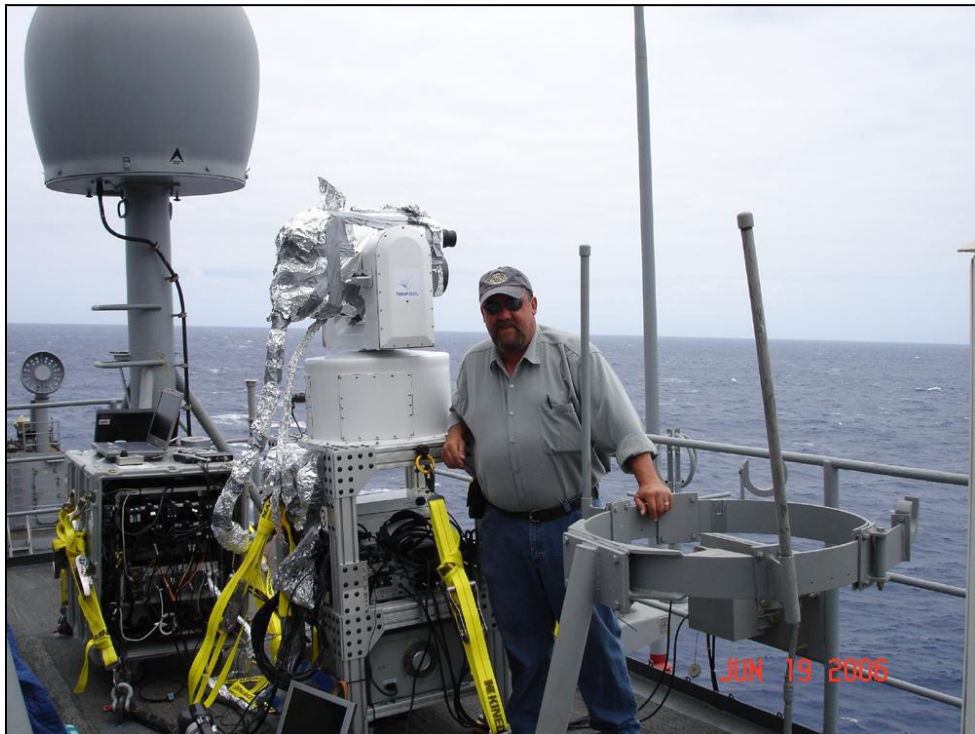
Figure 8: Novasol bistatic lasercomm terminal aboard the USS Denver
