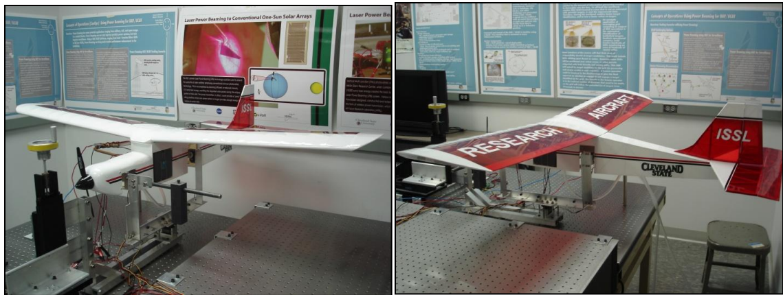
Figure 51: Gimbal rig with receiver, power electronics and MUAV
