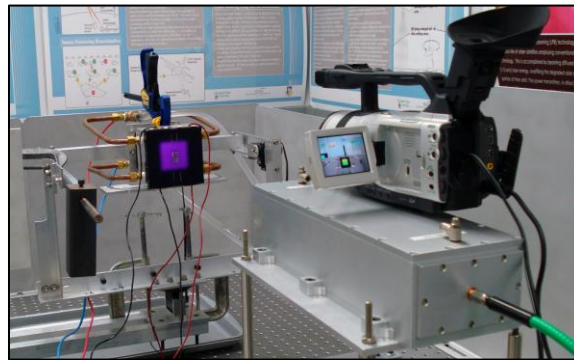
Figure 115: VMJ photovoltaic cell under pulsed illumination
