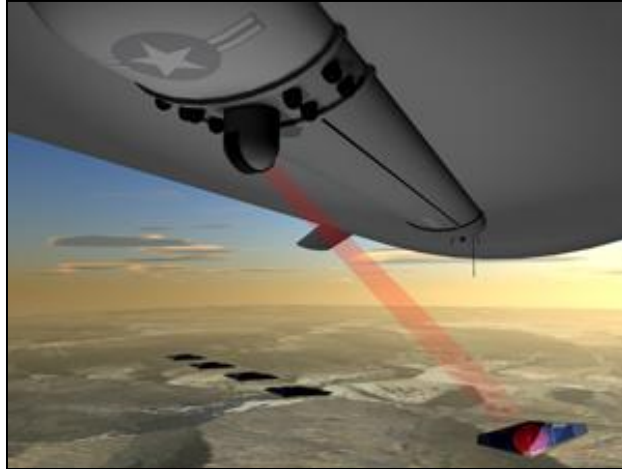
Figure 16: Airship optical link delivering power and/or communications
