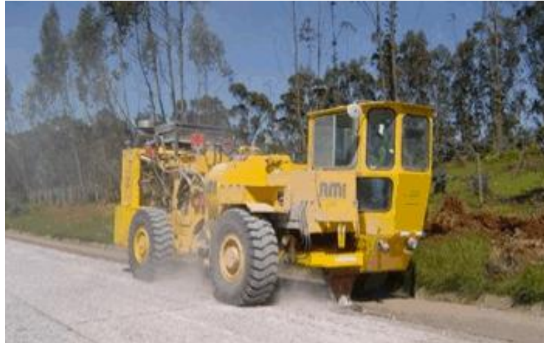
Figure 3 - Vehicle mounted resonance breaker (RMI Resonant Machines, 2011)
