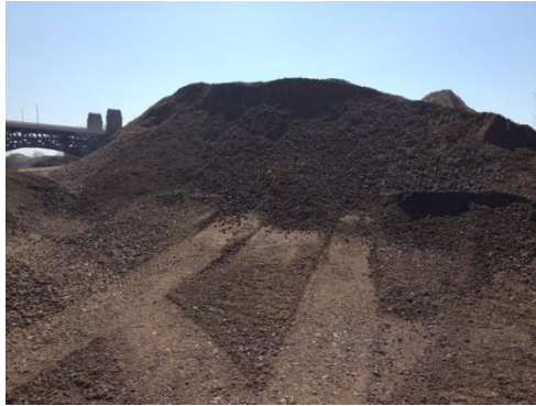
Figure 17 - "Dirty" #304 RCA base material
