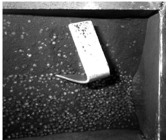
Figure 5.2: CB Separation from Pellet Prior to Feeding to extruder (Top View of Feed Hopper)
