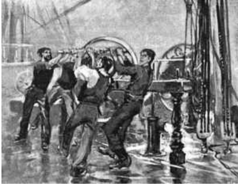
Figure 7 Illustration of sailors heaving a Downton pump. Reprinted from Operations of Downton Pump, in Wikipedia , (n.d.). Retrieved may 18, 2015, from en.wikipedia.org/wiki/Sea-shanty#/media/File:Downton_pump.tiff
