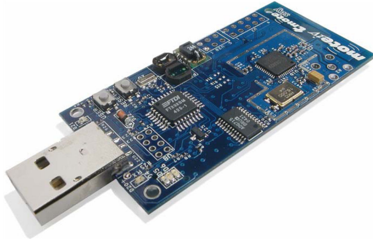
Figure 1: Tmote Sky iv Mote Device http://www.sic.rma.ac.be/Projects/WSN/tmote_sky.jpg
