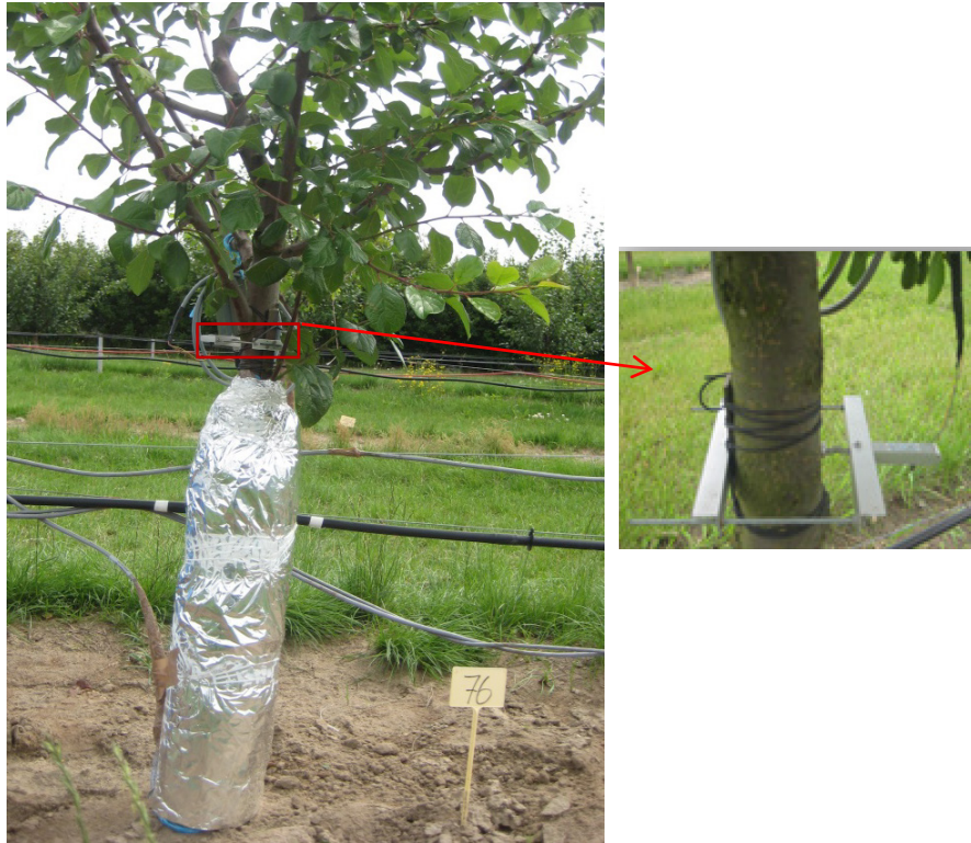
Fig. 5. Installation of dendrometer sensor to measure maximum daily shrinkage (MDS) together with dynage sensor for sap flow measurement (covered by aluminum foil; left figure).
