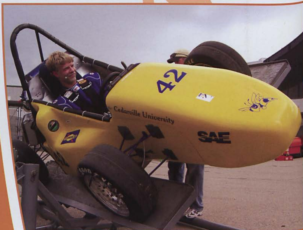
Dave Sampson rides in the car during the tilt test at the SAE competition: at 45 degrees no fluid can leak and at 60 degrees the car must not tip in this simulated 1G turn.
