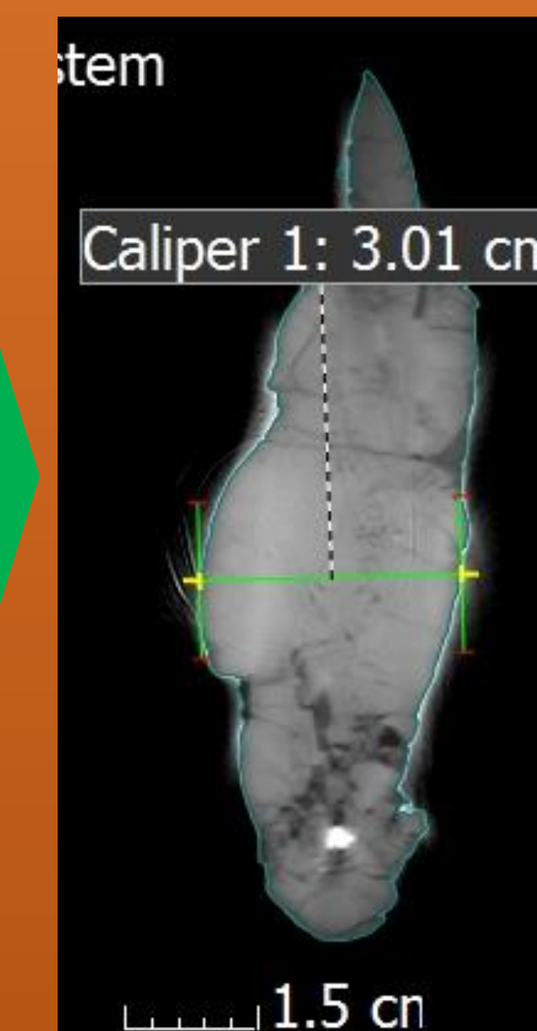
Figure 16: Single slice showing the use of the caliper tool in myVGL Viewer software.
