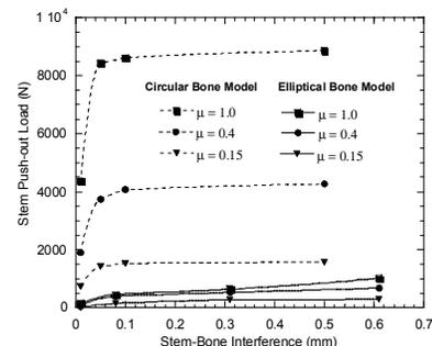
Fig. 3. Stem push-out load vs. stem-bone interference.
