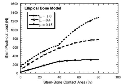
Fig. 2. Stem push-out load vs. contact area for elliptical bone canal.
