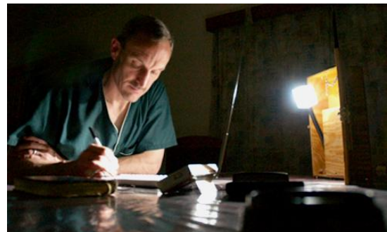
The student-designed reading light provides ample light on dark nights. The 9-LED light head draws so little current that a fully charged battery will last up to 60 hours.
