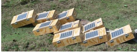
Solar lights being recharged in the sun. One hour of sunlight will provide one hour of use.
