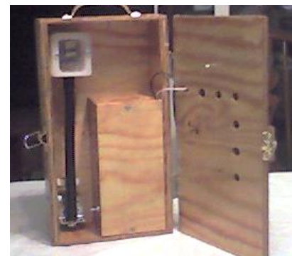
One version of the solar-recharged lights. This light had the light head inside the box mounted on a microphone gooseneck. The solar array is mounted on the top of the box, which being open, is not visible. These boxes were coated with polyester resin.
