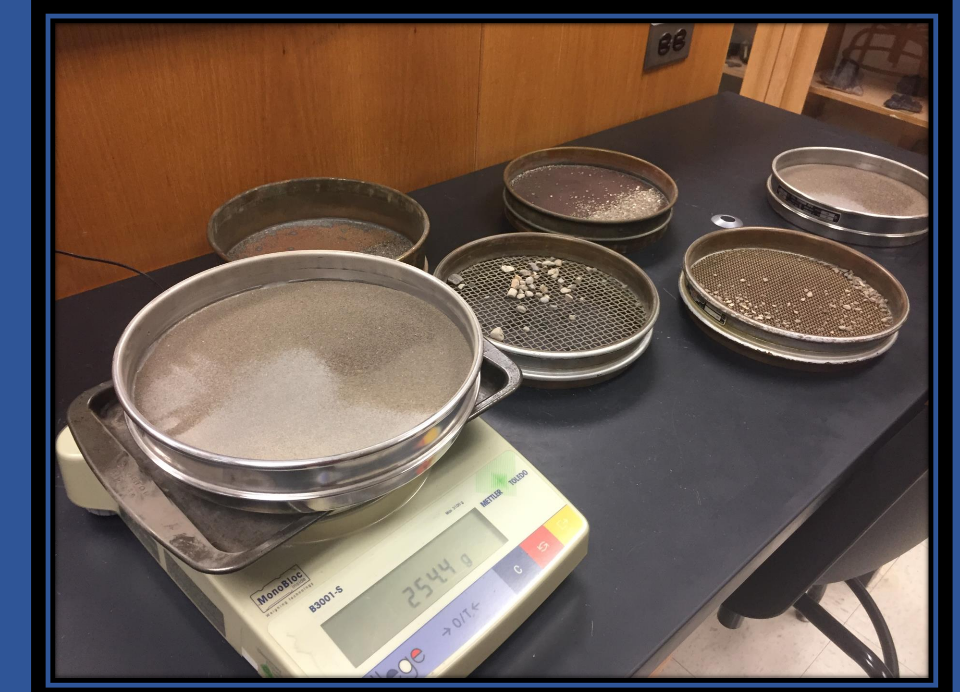
Sieves being weighed after the samples have been put through the shaker.
