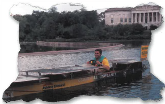
Above: Adam Yingling drove Cedarville's boat in the two-hour endurance event. The goal is to complete as many laps as possible. Solar cells provide some of the electricity to the motor. The strategy for this race is to drive as fast as possible to completely drain the batteries in exactly two hours. Going too fast will drain the batteries prematurely and going too slow will leave some charge in the batteries. The driver must monitor the current flow from the batteries and adjust the speed for optimum performance.
