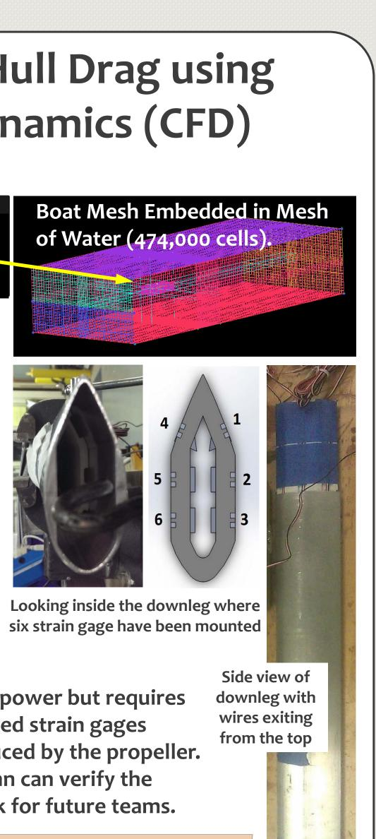
**CFD modelling requires massive amounts of computing power but requires** field measurements to validate the results. John mounted strain gages inside the downleg to measure thrust and torque produced by the propeller. At constant speed hull drag and thrust are equal, so John can verify the accuracy of his simulation. He has documented his work for future teams.
