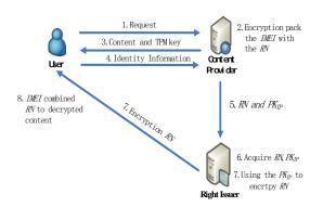
Figure 1: System architecture
