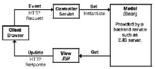
Figure1. M-V-C design pattern of eFramework
