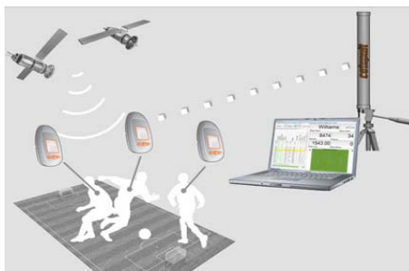
Figure 1: Components of the GPS monitoring process (Catapult 2009a).
