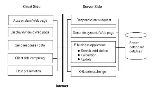
Figure 1. Client-Server Job Division in Service-Oriented Architectures
