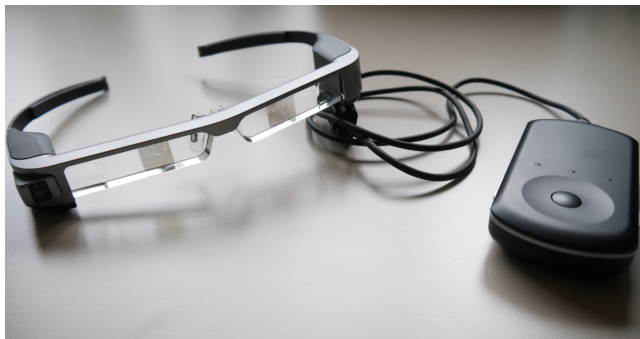
Figure 1. The Epson Moverio BT-300 HMD used for the Care Lenses (right: the handheld touch controller). Own image.
