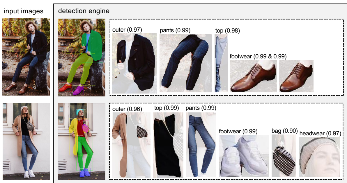
Figure 5. Demonstration of the detection engine (example images taken from zalando.com). The detected garment class names and probabilities are shown in the white box.
