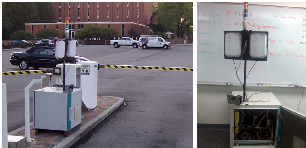
Figure 5. (a) Installation of the Parking Controller Portal at the Lot; (b) An Inside View of the Portal
