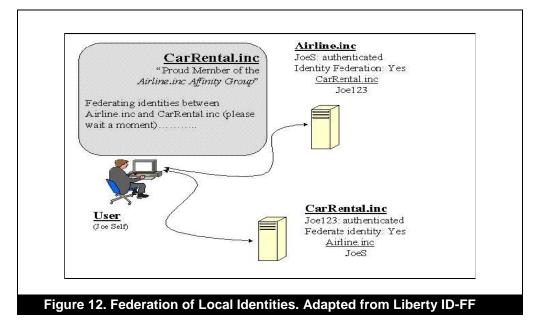
As illustrated in Figure 12, ID-FF provides for two types of user experience: identity federation and single sign on (SSO). SSO builds on identity federation and provides a relatively easy to use interface. Based on the ID-FF framework, the user logs into a website (an airline in this example) and is asked if they want to federate their airline identity with any other identity that they may have in the airline's circle. Upon consent, the identities are federated.
