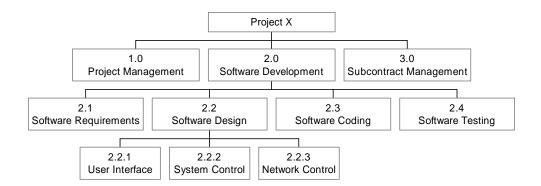
Figure 3. Work Breakdown Structure (WBS)
