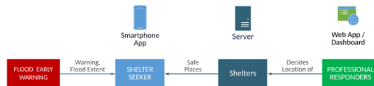
Fig. 2. Where should I go feature: both from the perspective of the smartphone app user (Shelter Seeker) and from the perspective of the dashboard users (Professional Responders);
