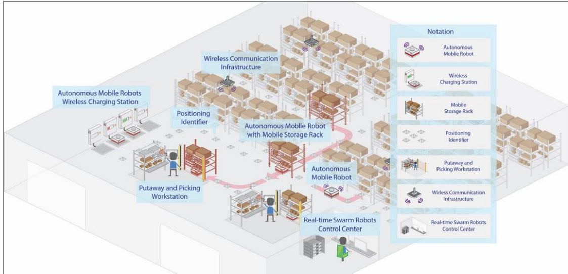
Fig 2. The overview of the IIoT-based Smart Robotic Warehouse Management System
