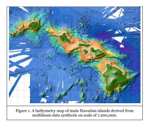
The geodetic parameters of the map in figure 1 include horizontal datum and ellipsoid are WGS-84 on Mercator projection and central Meridian of 0. The grid cell size is 50 meters with a 200 meter contour interval. The illumination is from the Northwest. Elevations for the islands are derived from USGS digital elevation model. Courtesy of Hawaii Mapping Research Group, University of Hawaii School of Ocean and Earth Science & Technology.
