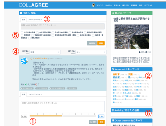
Fig. 1 Basic user-interface: each number shows characteristic functions explained in 3.1. Users can post their opinions in (3). (2) is a keyword extractor, and (1) is an automatic sentiment analyzer.
