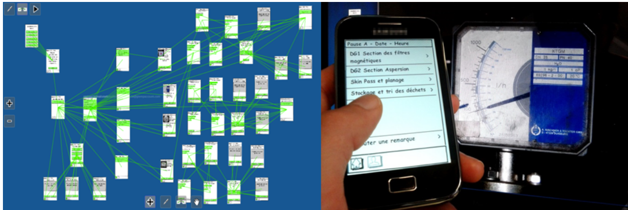
Figure 6. GAMBIT: Balsamiq Screens Interlinked to Form an Interaction Map (Left); Balsamiq Screens Running as Interactive Prototype on a Mobile Device (Right)
