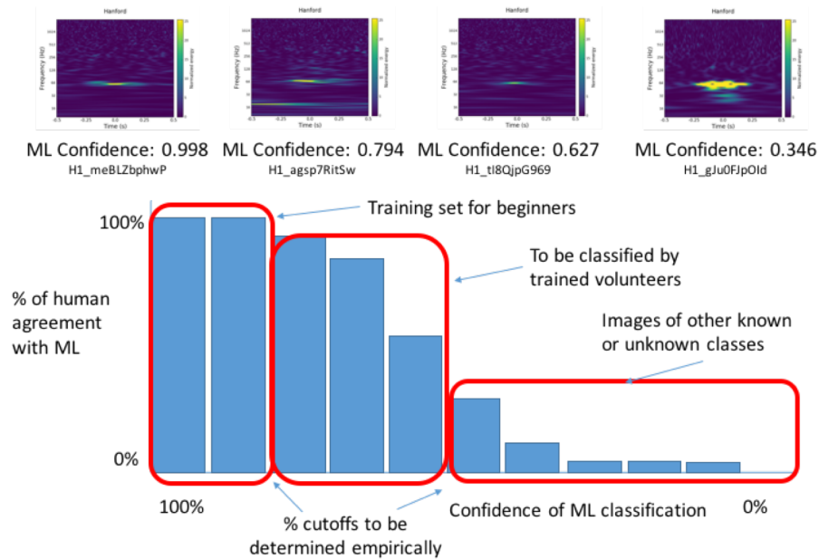
Figure 1. Relationship between ML confidence (x-axis) in a glitch belonging to a class and proportion of images assessed by human exports as belong to that class, with examples of glitches in each grouping.
