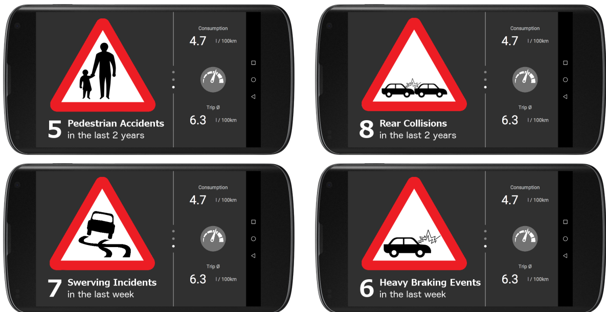
Figure 3. Examples of warning feedback provided by the information system. Top row: historic accident hotspot warnings. Bottom row: vehicle data hotspot warnings.
