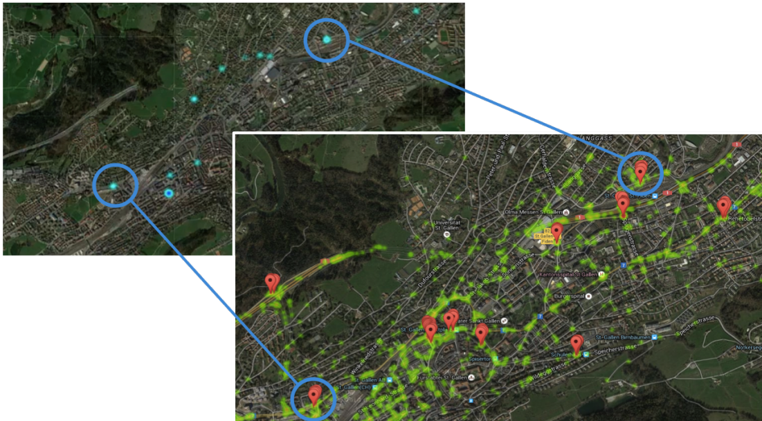
Figure 4. Preliminary results showing link between driving data and accident hotspots. Background image shows areas of heavy longitudinal deceleration in blue. Foreground image shows historic accidents in green and locations of accident hotspots with red markers.
