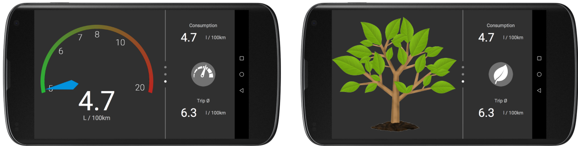
Figure 2. Non-warning feedback provided by the information system. From left to right: concrete fuel efficiency, abstract fuel efficiency.
