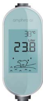
Figure 1. Snapshot of the information displayed by the smart shower meter. The screen can toggle to display energy use and the energy efficiency class in the upper part.
