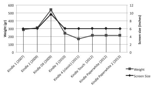
Figure 6: Comparison of weight and screen size of different versions of the Kindle
