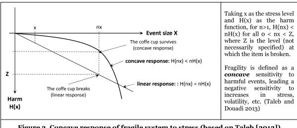
Figure 2. Concave response of fragile system to stress (based on Taleb [2012])
