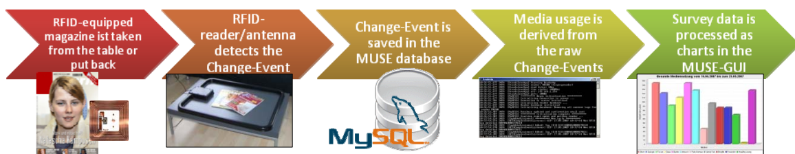
Figure 1. Sequence of the MUSE prototype functionality (own illustration)
