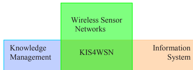
Fig. 1. The KIS4WSN system uses WSN to collect data, IS to store and manage data, and KM to extract and analyze data, and yield controls on WSN
