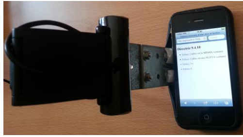
Fig. 1. Custom-made device used to record user interactions.
