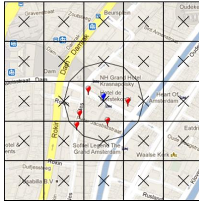
Figure 4. Illustrative box factor calculation: 100x100 meter grid with box center as reference point and POIs within 100m radius
