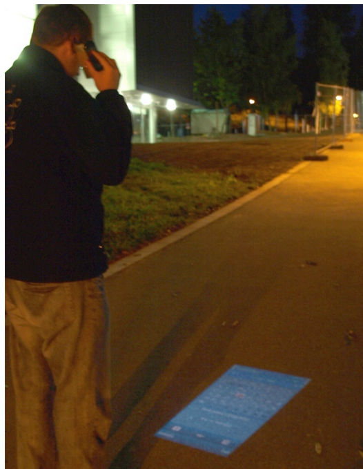
Figure 1 One handed interaction with a projector phone during a phone call: The user controls a cursor in the projection using a track pad on the back of the device.
