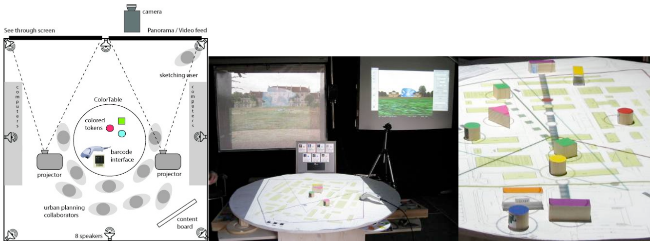
Figure 6: The technical setup inside the MR Tent is centered around the two projection walls and the ColorTable; representation of a scene on the physical map (right)
