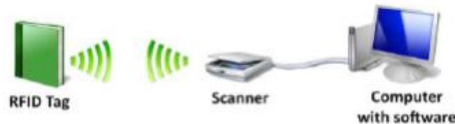
Figure 1. Component of RFID system
