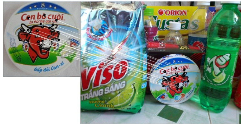
Figure 4. Detect a product logo in a query image using SURF features
