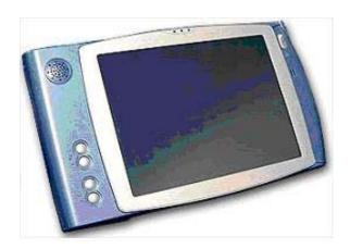
The 2.5lb AquaPad is a medium sized portable device centered around an 800x600 pixel TFT touch sensitive screen. The device is larger than a PDA, but smaller than a laptop.
