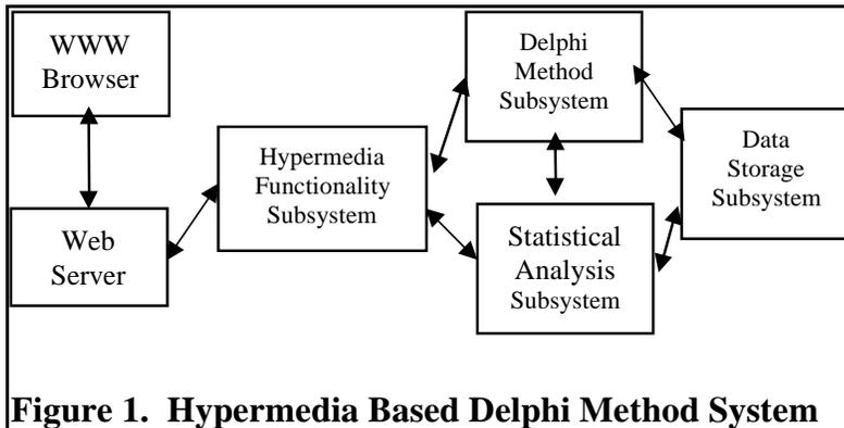
**Figure 1. Hypermedia Based Delphi Method System**
